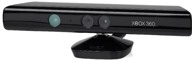
Kinect.v1: structured light
