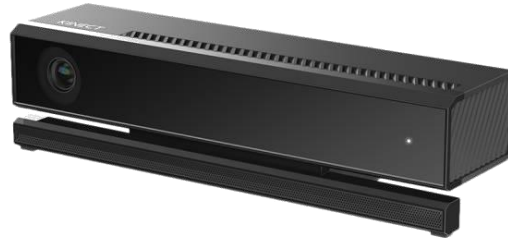
Kinect.v2: time of flight
