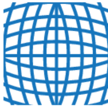
Positive radial distortion "barrel"
